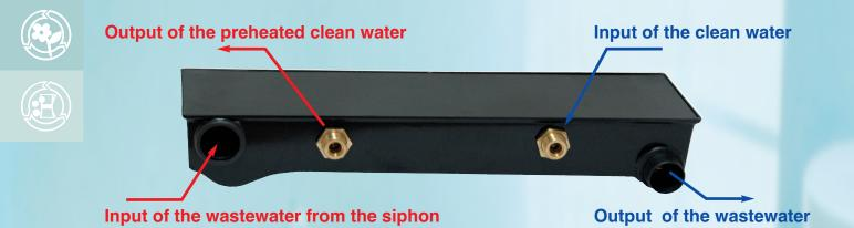
The shower exchanger NELA is intended for the wastewater recovery in the bathrooms.
