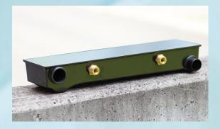
**The NELA Shower Exchanger** is constructed to recover heat from used shower water. Warm water from the shower drain flows through the NELA Shower Exchanger and pre-warms the cold clean water by approximately 12 degrees Celsius prior to entering the thermostatic mixer tap. The amount of hot water required is therefore lowered, thus in turn saving more than 45% of energy used when compared to conventional shower water heating.
