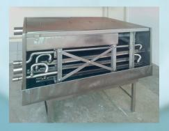
We also specialize in design and production of dedicated waste-water heat recovery exchangers which do not need pre-conditioning or filtering of the dirty waste water. Our range of products include **SUP Exchangers** for large industrial use, such as
